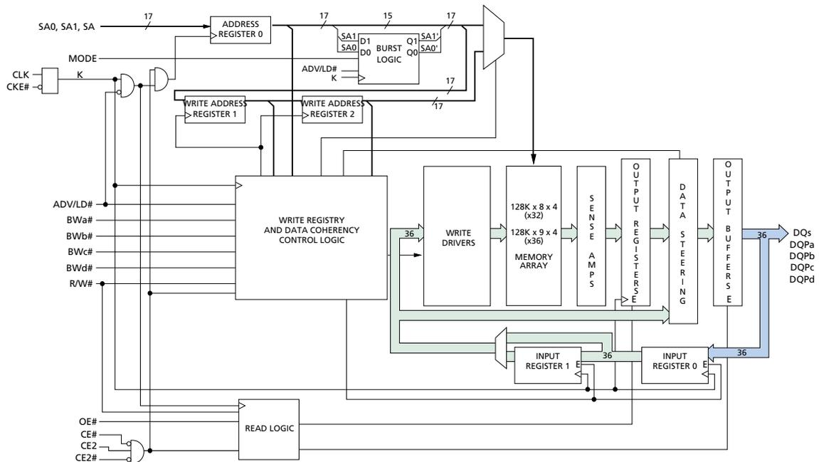
**NOTE:** Functional block diagrams illustrate simplified device operation. See truth tables, pin descriptions, and timing diagrams for detailed information.
