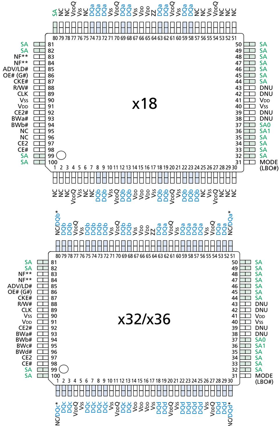
\*No Connect (NC) is used on the x32 version. Parity (DQPx) is used on the x36 version.
